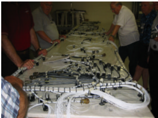
Some of the 5 miles of wire in the DC 3
