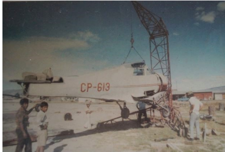
Upper left: Stag stored on a farm just outside of Cochabamba for about one year while paperwork was done for exportation. Right: Building pallet for fuselage. (All done with Bolivian mahogany.) Lower left: Hand-crank crane to lift the fuselage onto the pallet.
