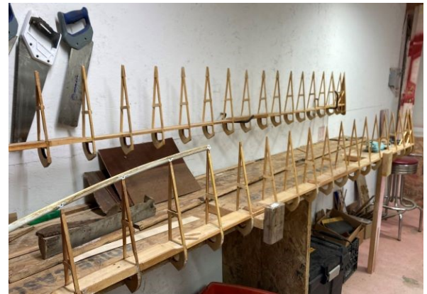
Above: The original fuel valve. Right: Restoration of the wing components.
