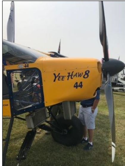
These are pics of Steve Henry and Yee-Haw. He is a short takeoff and landing (STOL) aircraft champion. This airplane is powered by a three-cylinder turbocharged Yamaha snowmobile engine developing several hundred horsepower at 9,000 RPM.
