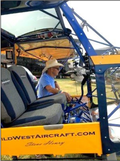
These are pics of Steve Henry and Yee-Haw. He is a short takeoff and landing (STOL) aircraft champion. This airplane is powered by a three-cylinder turbocharged Yamaha snowmobile engine developing several hundred horsepower at 9,000 RPM.
